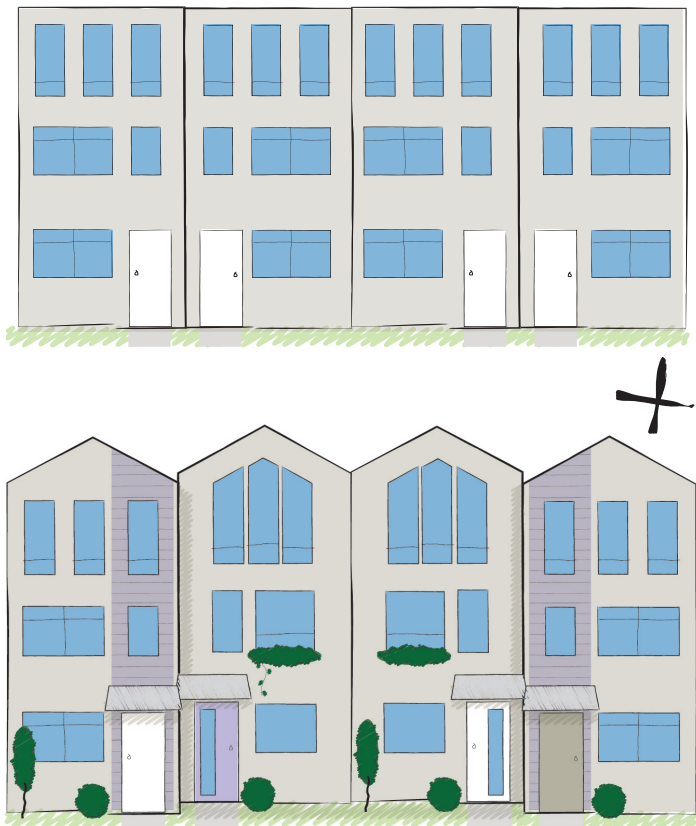
DIAGRAM 10 - COMPLEMENTARY DESIGN FEATURES AND RECESSED BUILDINGS CONTRIBUTE TO ATTRACTIVE AND LEGIBLE BUILDING DESIGN
