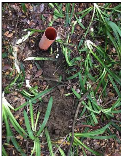
Figure 2 - Soil extracted during hand augering
