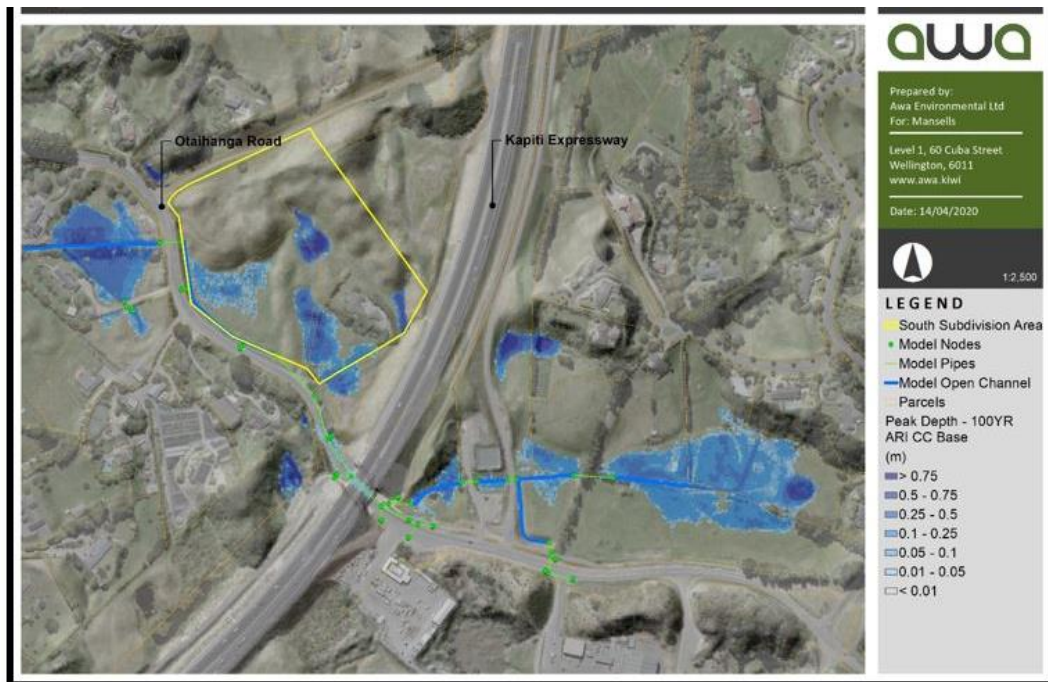
Figure 6: 100-year ARI CC peak inundation depths- base scenario for the southern part of the site (Awa 2021).
