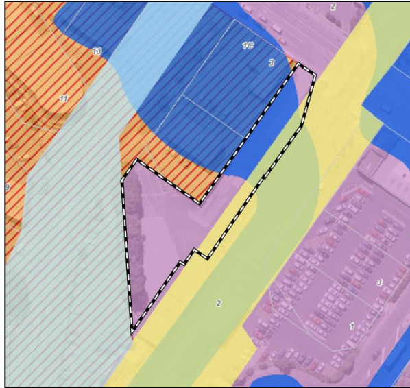
Figure 6 – Zoning of the site at. Purple denotes the Industrial Service Zone, Yellow donates the Railway Designation and blue shows the ponding flood hazard on the site.
