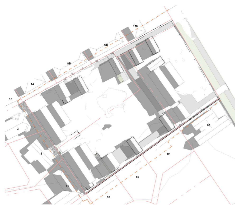
PERMITTED BASELINE - SOLAR SHADING - AUTUMN SOLSTICE 9AM SCALE @ A3 -1 : 1300 | SCALE @ A1 - DOUBLE SCALE
