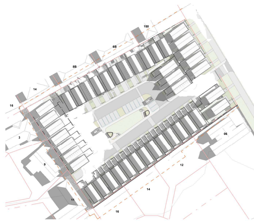
PROPOSED - SOLAR SHADING - AUTUMN SOLSTICE 9AM SCALE @ A3 -1 : 1300 | SCALE @ A1 - DOUBLE SCALE
