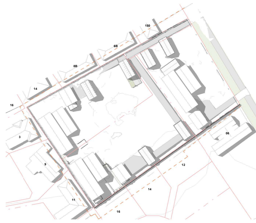
PERMITTED BASELINE - SOLAR SHADING - SUMMER SOLSTICE 3PM SCALE @ A3 -1 : 1300 | SCALE @ A1 - DOUBLE SCALE
