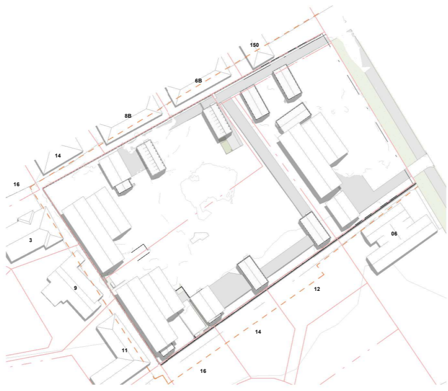
PERMITTED BASELINE - SOLAR SHADING - SUMMER SOLSTICE 12PM SCALE @ A3 -1 : 1300 | SCALE @ A1 - DOUBLE SCALE
