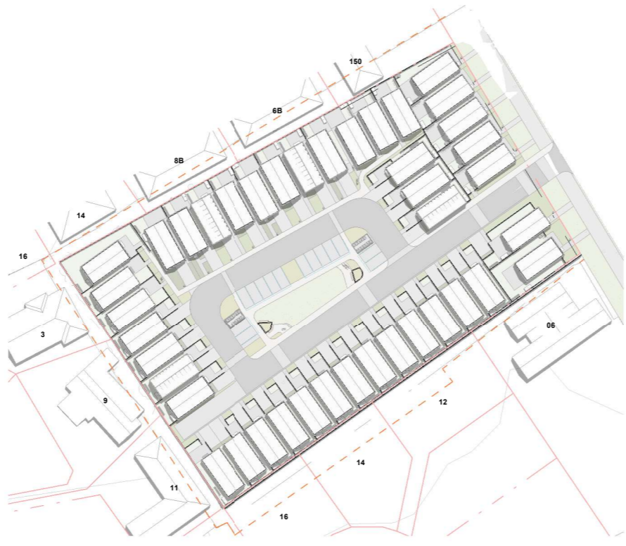
PROPOSED - SOLAR SHADING - SUMMER SOLSTICE 12PM SCALE @ A3 -1 : 1300 | SCALE @ A1 - DOUBLE SCALE
