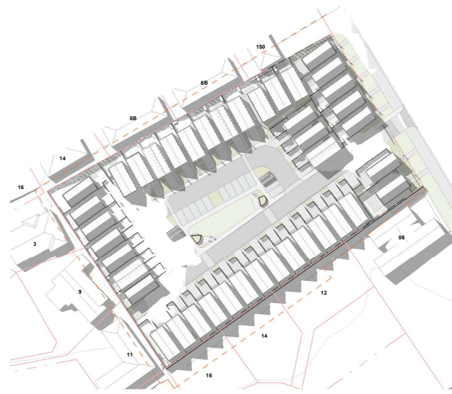
PROPOSED - SOLAR SHADING - AUTUMN SOLSTICE 3PM SCALE @ A3 -1 : 1300 | SCALE @ A1 - DOUBLE SCALE
