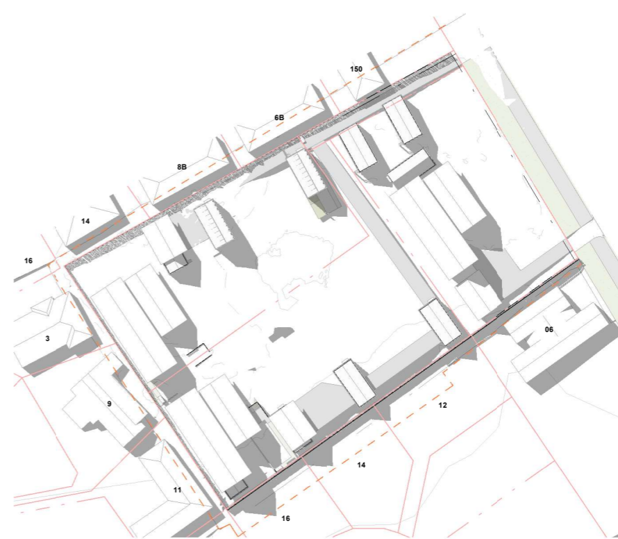
PERMITTED BASELINE - SOLAR SHADING - AUTUMN SOLSTICE 3PM SCALE @ A3 -1 : 1300 | SCALE @ A1 - DOUBLE SCALE
