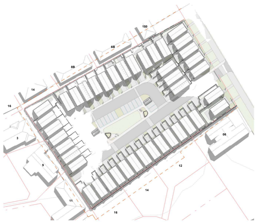
PROPOSED - SOLAR SHADING - AUTUMN SOLSTICE 12PM SCALE @ A3 -1 : 1300 | SCALE @ A1 - DOUBLE SCALE
