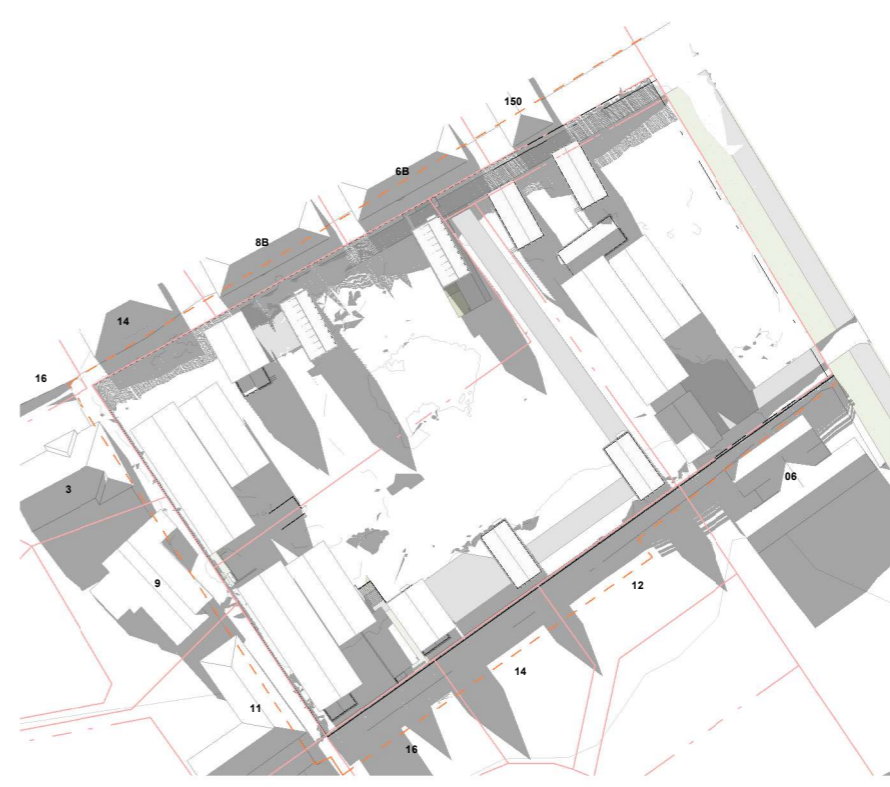
PERMITTED BASELINE - SOLAR SHADING - WINTER SOLSTICE 3PM SCALE @ A3 -1 : 1300 | SCALE @ A1 - DOUBLE SCALE
