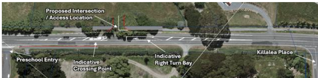
Figure 14: Concept design for a new intersection on Ratanui Road
