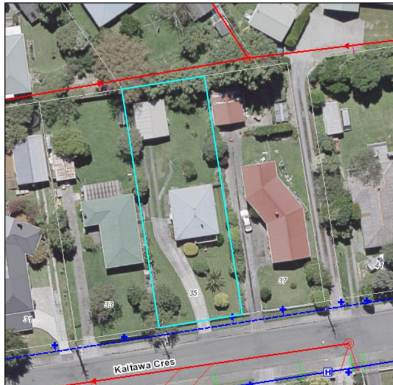
Figure 6: Existing and surrounding services. Dark blue = water, red = sewer and pink = private connections
