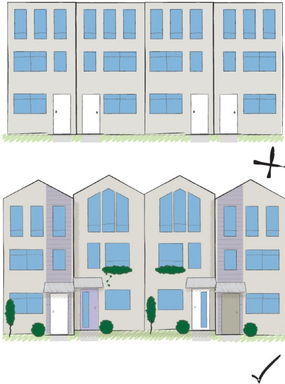
Diagram 10 - Complementary design features and recessed buildings contribute to attractive and legible building design
