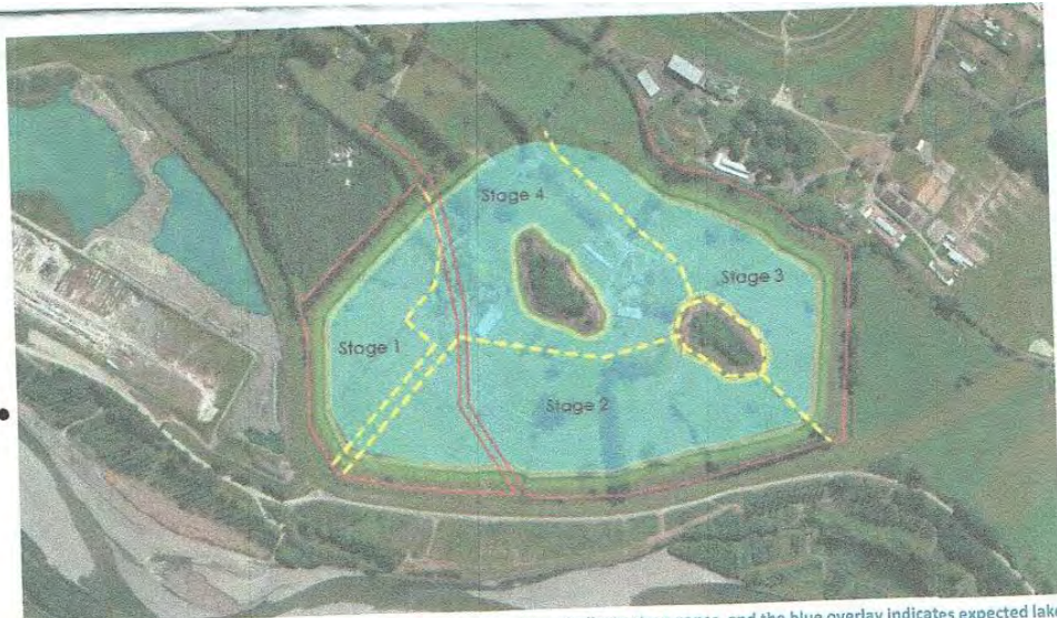
Figure 1: Overview of the Ashford Park Quarry site. Yellow dashed lines indicate stage zones, and the blue overlay indicates expected lake extent. Green area is the approximate riparian area, however the margins will differ from those shown. Map is north-facing.
