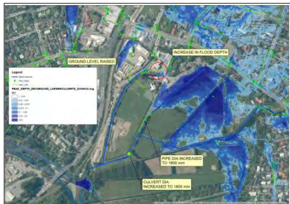
Figure 13: Modelled peak depths of ponding post-development within submitters land of Waikanae East (source: Prepared by AWA Environmental Ltd for Goodman Holdings Ltd - 2017)
