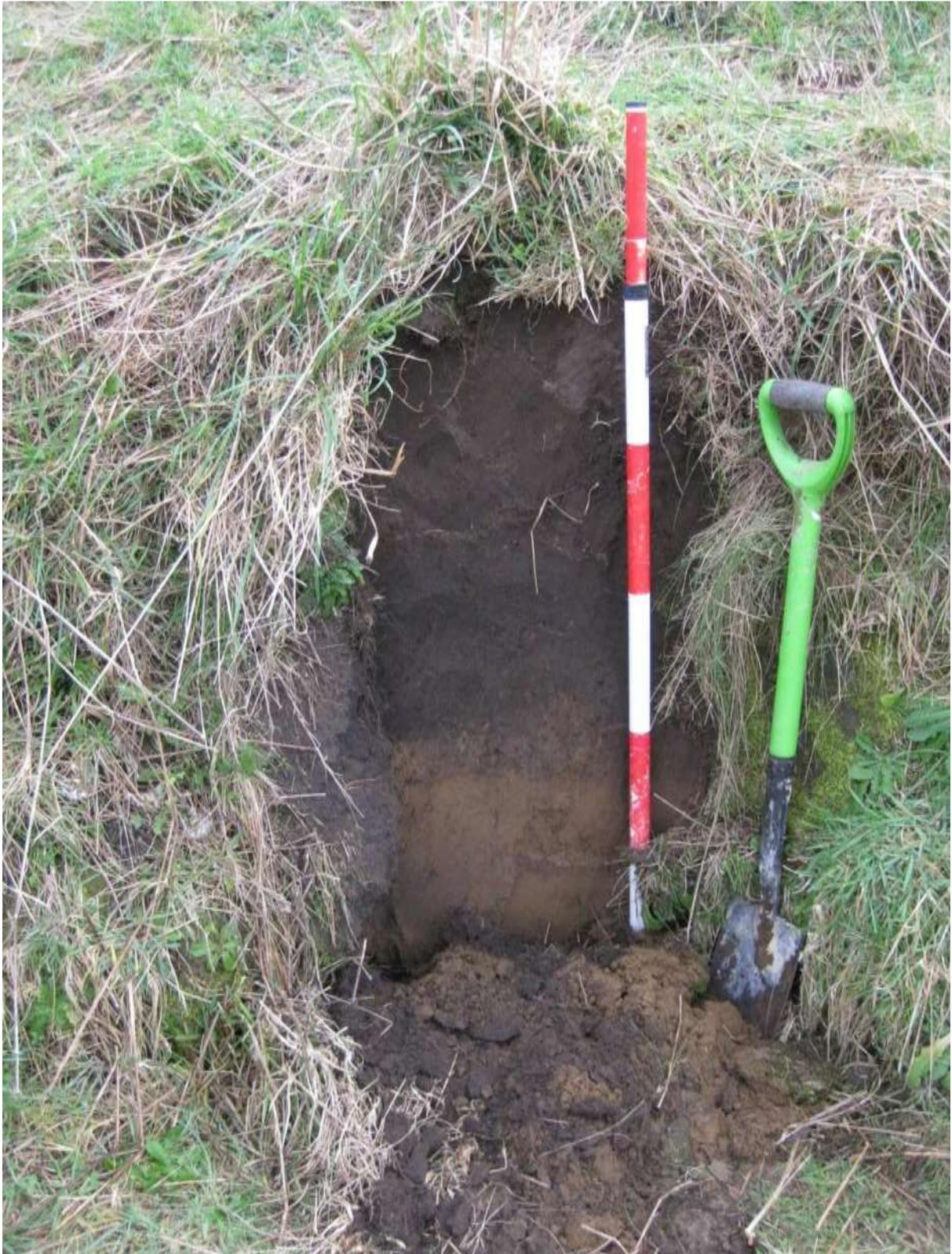
Fig. 13. TP 1 profile of cattle scrape (Section 24). Unexpectedly deep (70 cm) topsoil (dark layer) suggests disturbances on the slope above and steady slope wash over the years.
