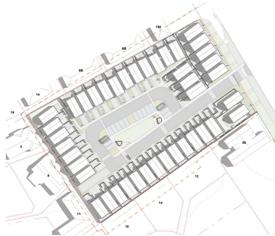
PROPOSED - SOLAR SHADING - SUMMER SOLSTICE 9AM SCALE @ A3 -1 : 1300 | SCALE @ A1 - DOUBLE SCALE
