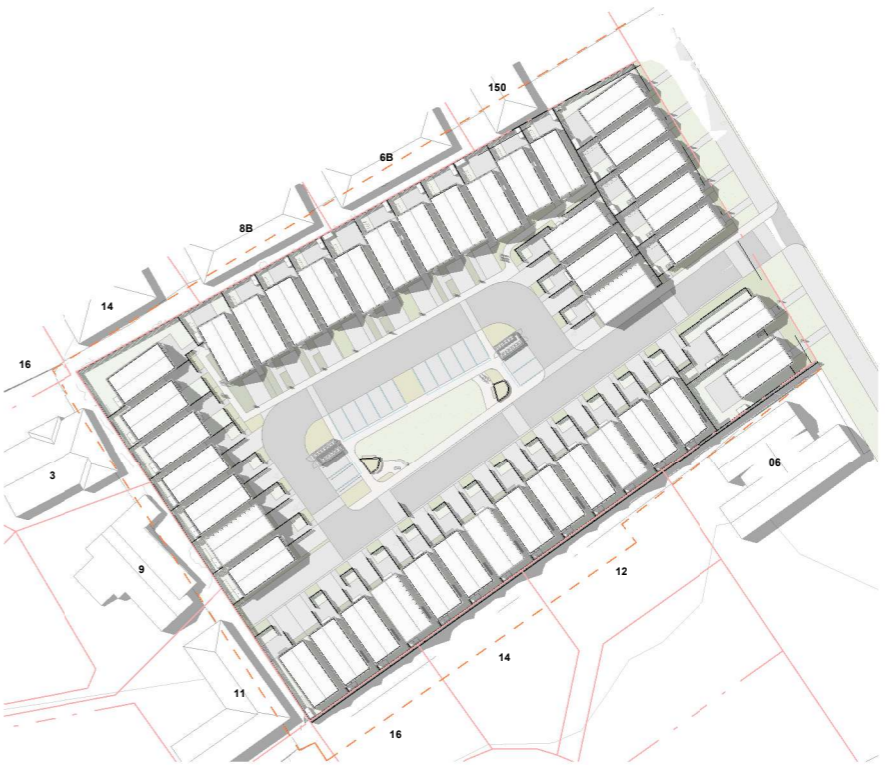
PROPOSED - SOLAR SHADING - SUMMER SOLSTICE 3PM SCALE @ A3 -1 : 1300 | SCALE @ A1 - DOUBLE SCALE
