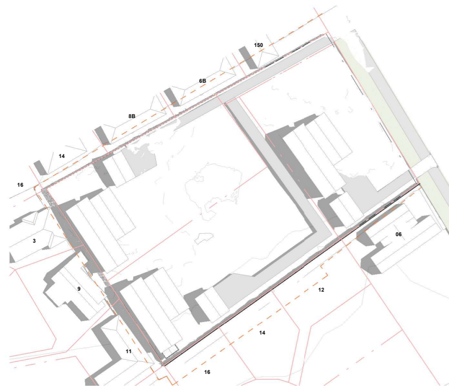
PERMITTED BASELINE - SOLAR SHADING - SUMMER SOLSTICE 9AM SCALE @ A3 -1 : 1300 | SCALE @ A1 - DOUBLE SCALE
