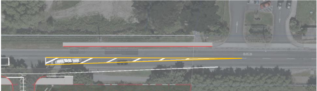
Figure 4: Indicative Taper for 60km/h Design Speed (Orange)
