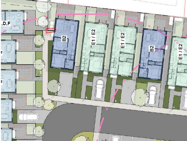
Figure 1: Unit 19 (B2 on left) has its entrance on a secondary pedestrian path. Side yard entrance could be changed to western side (marked in red) to improve legibility.
