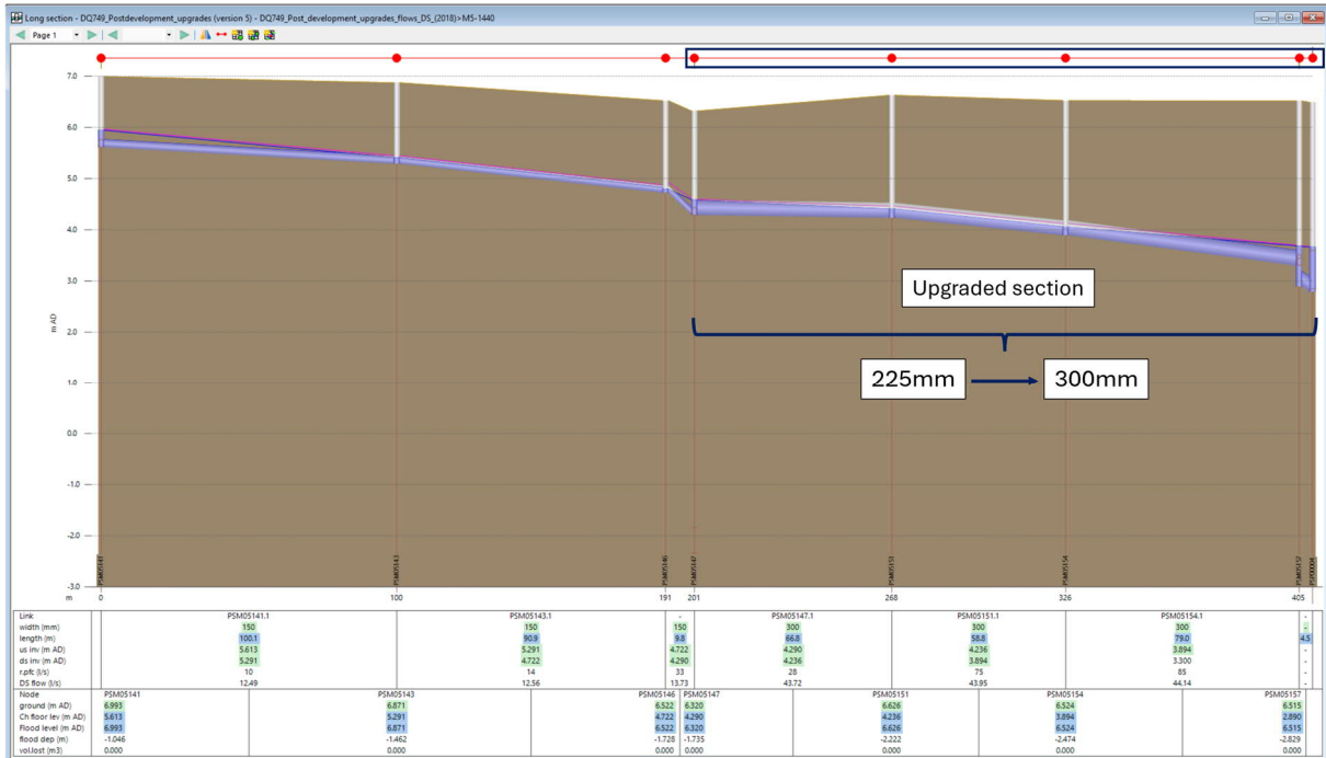
Figure 5: Post-development flows to PSP0004 with upgrades - 5-year ARI design storm, long section
